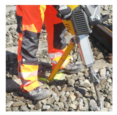
Practical shock absorber Supports the user in guiding the off track tamping machine.
