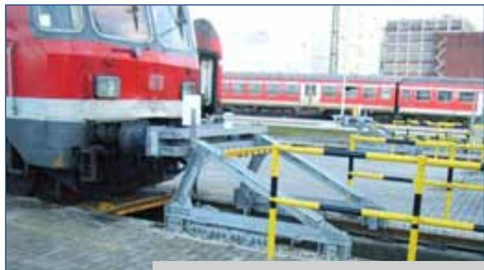
Friction buffer stop on a pit in a workshop
