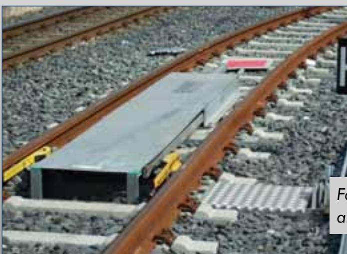
Folding drag shoe system including manual device and additional friction device
