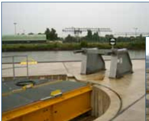
Standard type FP200HP with hydraulic friction device
