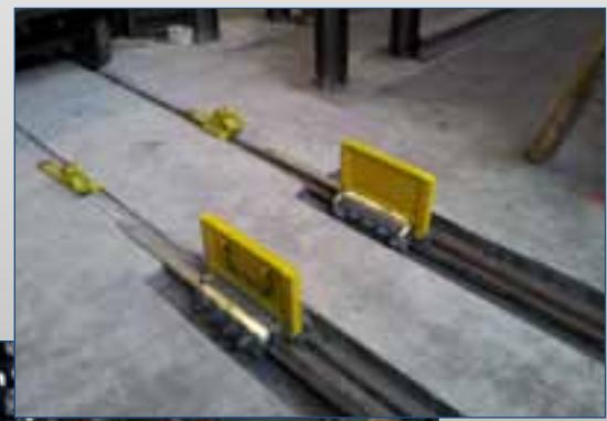
Friction wheel stop, retractable design including cover plates for sliding
