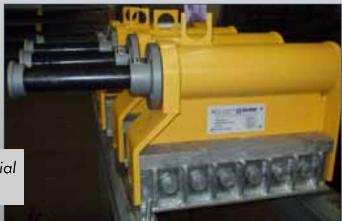
End stop design for impact height of 1.9m
